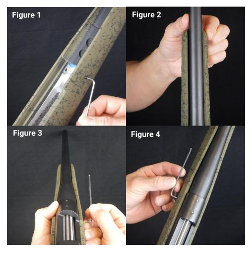
Our Pro-Center® technology is a major advancement in firearm stocks. This technology allows anyone to center the barrel in the stock, regardless of dimensional variances in the barreled action. If you are unable to center the barrel in the stock, the tolerances of your barreled action may be out of specification. Please contact your barreled action manufacturer before making any modifications.
